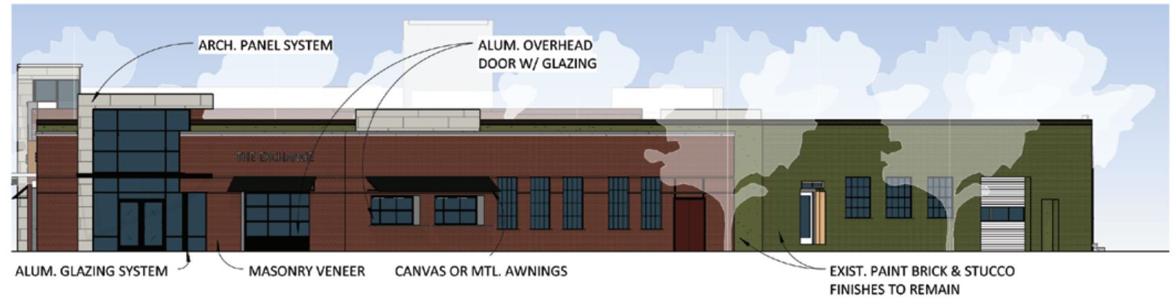
SOUTH BUILDING SOUTH ELEVATION PDR SUBMITTAL
